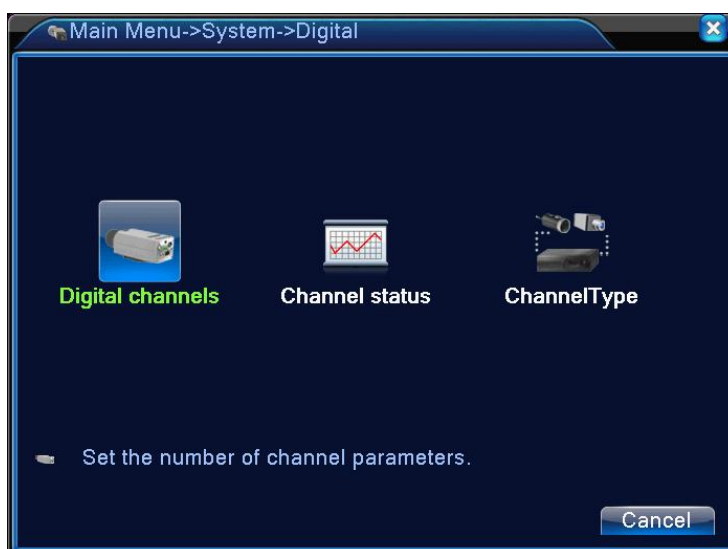
Pic 4.34 channel manage interface
