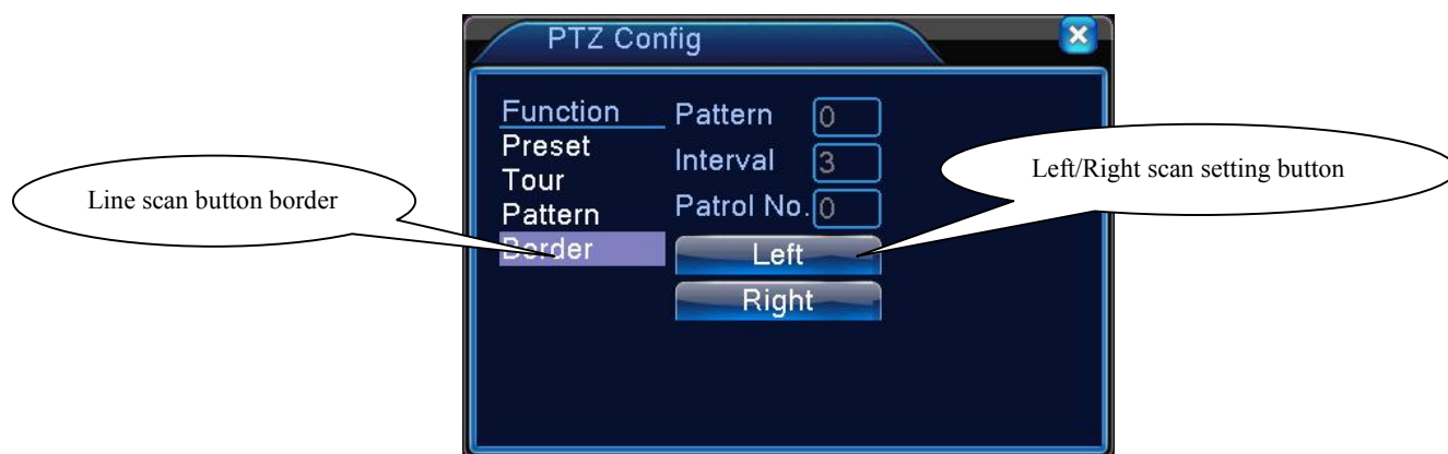
Pic 3.13 Boundary Scan Setup
